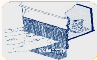
Foundation with wire mesh
